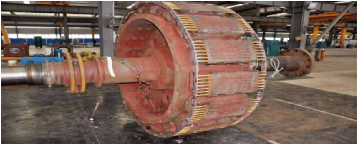
● 晋煤冀衡化肥TK2550-18/2600 2550KW 10KV 压缩机电机转子笼条大修更换
